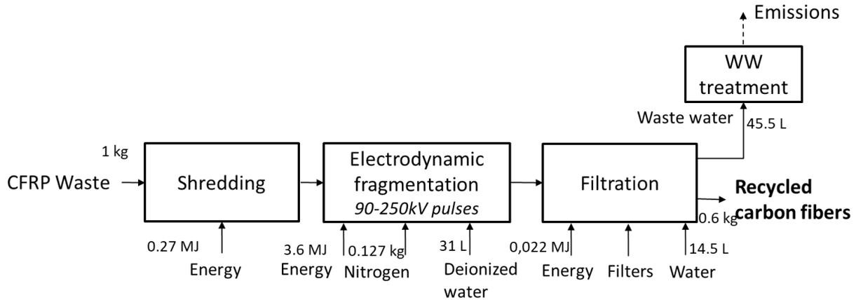
Figure 5: Representation of the electrodynamic fragmentation process
