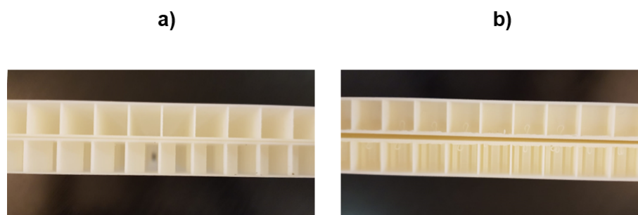
Figure 8: The 3D-printed panels side-view following the standard (up) and optimised(down) designs in: a) Fig. 2 - Double-Wall panel with mechanical links; b) Fig. 5 - Sandwich panel with rectangular core.
