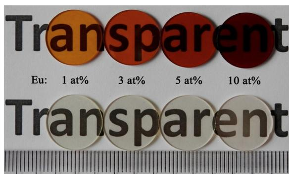
Fig. 35. Photographs of the as-sintered (above) and thermally annealed (below)  $\text{Eu}^{3+}$ -doped  $\text{La}_{0.8}\text{Gd}_{1.2}\text{Hf}_2\text{O}_7$  ceramics. Reused from [394], Copyright © 2017, Elsevier.
