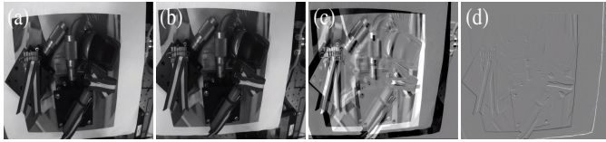
Fig. 14: [Experiment - 3D Scene] - Achievement of the positioning task using a 3D object. (a): I^* , (b): I , (c): the initial error and (d): the final one.
