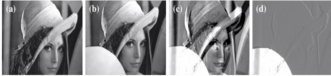
Fig. 11: [Experiment - Partial Occlusions] - visual servoing task achievement under partial occlusions. (a) I^* , (b) I , (c) initial image difference, and (d) final one.
