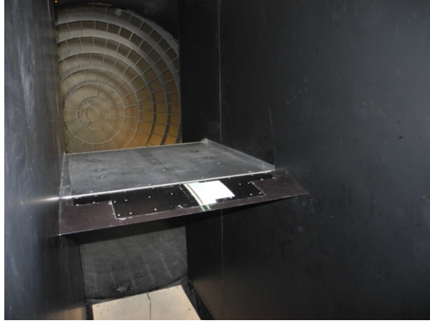
Fig. 1 Flat plate model with hinged slotless flap in the L1 wind tunnel.
