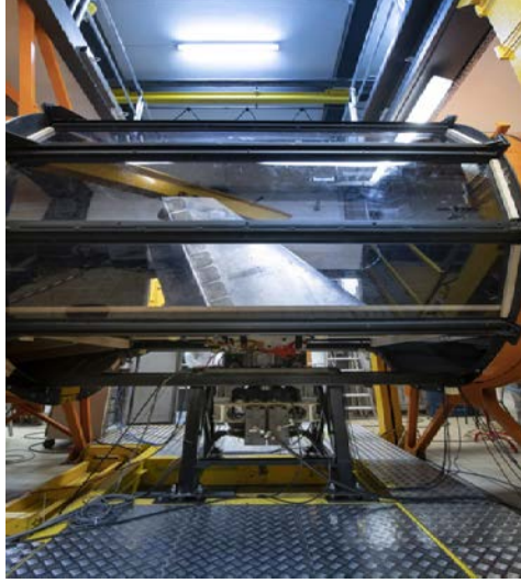
Fig. 15 Model set-up with balance.
