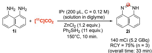
**Scheme 5.** Production of perimidine **2i**. The RCY value is mean value and was estimated from trapped  $[^{11}\text{C}]\text{CO}_2$  within the reactor and are decay-corrected from end of  $[^{11}\text{C}]\text{CO}_2$  trapping inside reactor.
