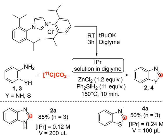
**Scheme 4.** Cyclization reactions with home-made solution of **IPr**. Radiochemical yields are mean values and were estimated from trapped  $[^{11}\text{C}]\text{CO}_2$  within the reactor and are decay-corrected from end of  $[^{11}\text{C}]\text{CO}_2$  trapping inside reactor.
