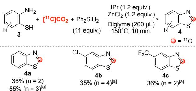
**Scheme 2.** Cyclizations of aminobenzenethiols with  $[^{11}\text{C}]\text{CO}_2$ . Radiochemical yields are mean values and were estimated from trapped  $[^{11}\text{C}]\text{CO}_2$  within the reactor and are decay-corrected from end of  $[^{11}\text{C}]\text{CO}_2$  trapping inside reactor. [a] diglyme volume = 100  $\mu\text{L}$ .
