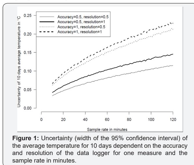
**Figure 1:** Uncertainty (width of the 95% confidence interval) of the average temperature for 10 days dependent on the accuracy and resolution of the data logger for one measure and the sample rate in minutes.
