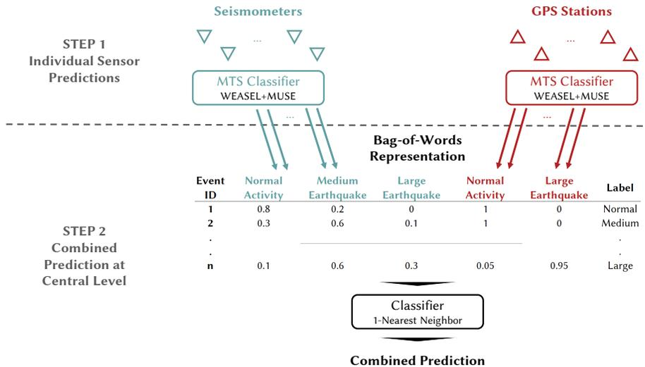
Figure 1: Distributed Multi-Sensor Earthquake Early Warning Algorithm (DMSEEW).
