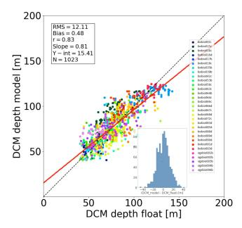
**Figure 2.** Match-up diagram comparing DCM depth obtained from BGC-Argo float data versus REF model results. Each dot corresponds to a weekly profile. The red line depicts the linear regression between data and model values, defined by its slope and intercept (Y-int) shown in the box. Units of RMSD, bias, and Y-int are in metres. The correlation coefficient r is significant, with p value < 0.005. The bottom sub-figure shows the residuals' histogram.
