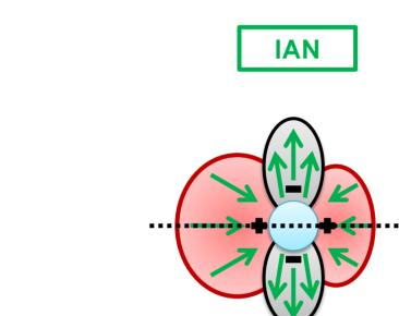
Uniform distribution of p<sub>rad</sub> acts Non symmetric distribution of like a pressurized environment p<sub>rad</sub> along the acoustic axis  $F_{rad} = 0$
