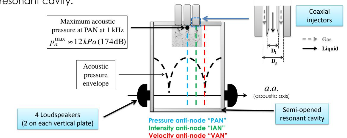
Anti-node: spatial location where the amplitude of fluctuations of the considered acoustic quantity (e.g. pressure, velocity or intensity) is
