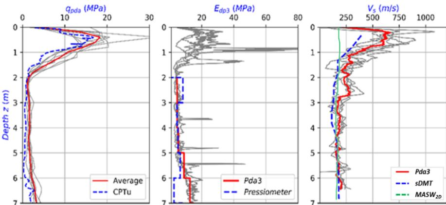
Figure 3. In-situ test campaign: comparative tests. (a) Peak resistance profiles  $q_d$ : Panda3® vs CPTu; (b) Module profiles ( $E_{Kd_{min}} / E_M$ ): Panda 3® vs PMT, and (c) Shear wave velocity profile: Panda 3®, MASW2D and sDMT. A very good correspondence is observed between the different tests.
