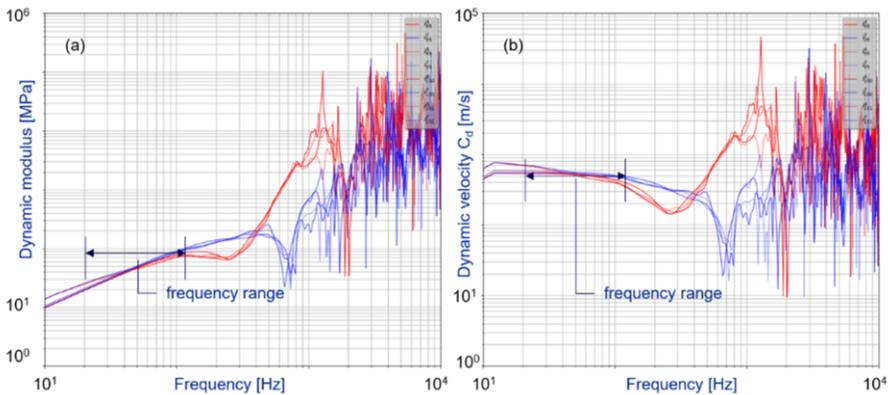
**Figure 1:** Example of the evolution of the dynamic modulus  $E_{Kd}$  (a) and the compression wave velocity  $V_p$  as a function of frequency  $f$ . Red lines represent the signals recorded at the top (measurement section), while the blue lines represents the signal reconstructed at the bottom level (penetrometer tip)
