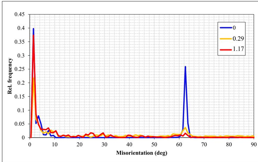
Fig. 13. Evolution of misorientation angles during thermal cycling test. Twin boundaries tend to disappear as it can be noticed with the yellow ( $D_{solder} = 0.29$ ) and red curves ( $D_{solder} = 1.17$ ) which do not exhibit a high peak around  $60^\circ$ . (For interpretation of the references to colour in this figure legend, the reader is referred to the web version of this article.)
