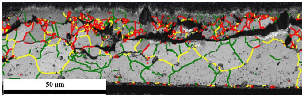
Fig. 9. High angle grain boundaries near crack in the high strain region beneath the R2512 component for  $D_{\text{solder}} = 0.29$  (green:  $0^\circ$ – $15^\circ$ , yellow:  $15^\circ$ – $45^\circ$ , red:  $> 45^\circ$ ). (For interpretation of the references to colour in this figure legend, the reader is referred to the web version of this article.)
