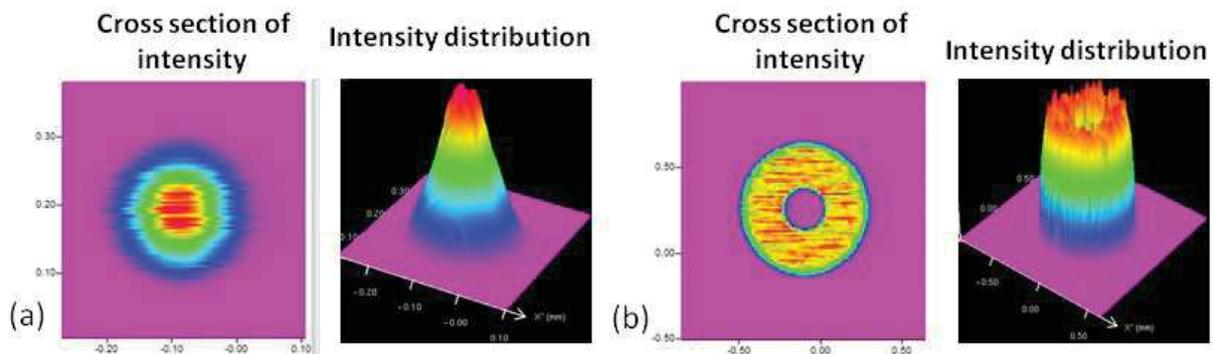
Figure 2: Intensity distributions at the focal point with (a) the 100  $\mu\text{m}$  core fiber (500 W,  $\Phi=150 \mu\text{m}$ ), (b) the 400  $\mu\text{m}$  outer fiber (500 W,  $\Phi=150 \mu\text{m}$ ) measured with a Primes Focus monitor device.
