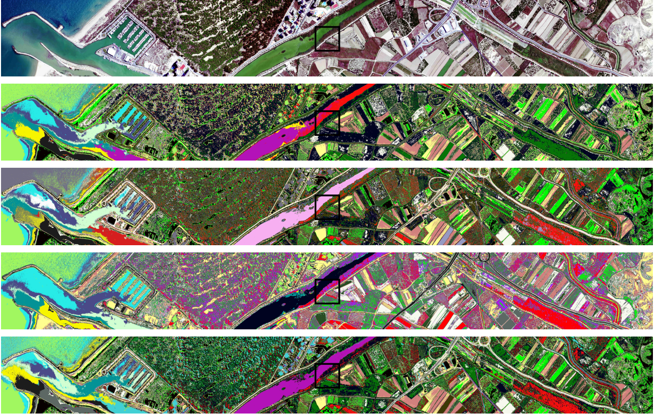
Figure 9. Clustering results using NN-DB methods on a very large HSI ( 8192 \times 960 pixels, 62 bands). From top to bottom: Guardamar hyperspectral image (Color composite, bands 30, 20, 10); ModeSeek; knnDPC ; knnClust-WM; GWENN-WM.
