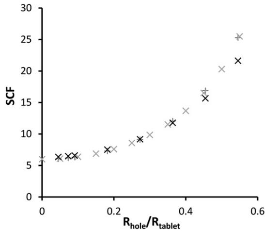
**Fig. 3.** SCF as a function of the ratio between the hole radius ( $R_{\text{hole}}$ ) and the tablet radius ( $R_{\text{tablet}}$ ): analytical results (x) and FEM results for the standard (+) and flattened (\*) geometry.
