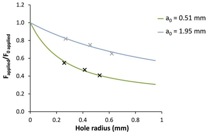
**Fig. 7.** Application of the average stress criterion. The graph represents the ratio between the force needed to break a compact with a hole and the force needed to break a compact without a hole as a function of the hole radius. Continuous lines are obtained according to Eq. (14) for several values of  $a_0$ . Marks represent the experimental values: (x) SDLac and (x) aCP.
