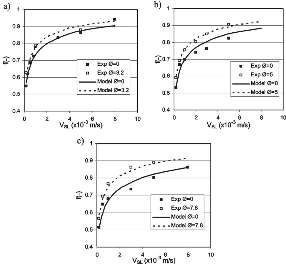
**Figure 8.** Effect of silicon carbide fines: alumina particles of (a)  $d_v = 2.85 \times 10^{-3}$  m, (b)  $d_v = 4.5 \times 10^{-3}$  m, (c)  $d_v = 7 \times 10^{-3}$  m. Cases 6 and 13–17 from Table 3 ( $\phi = 0$  corresponds to the bed without fines,  $\phi = d_v/d_{SiC}$  otherwise).
