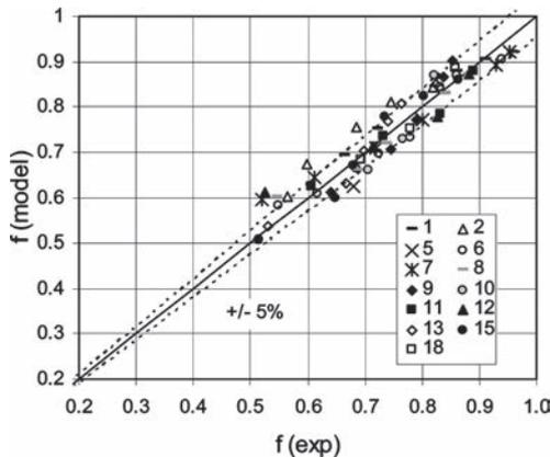
**Figure 9.** Parity diagram for wetting liquid/alumina systems. See Table 3 for experimental conditions.
