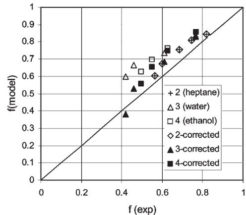
**Figure 10.** Parity diagram of original and modified correlation for heptane, ethanol, and water (data from Baussaron et al.<sup>11</sup>). See Table 3 for experimental conditions.
