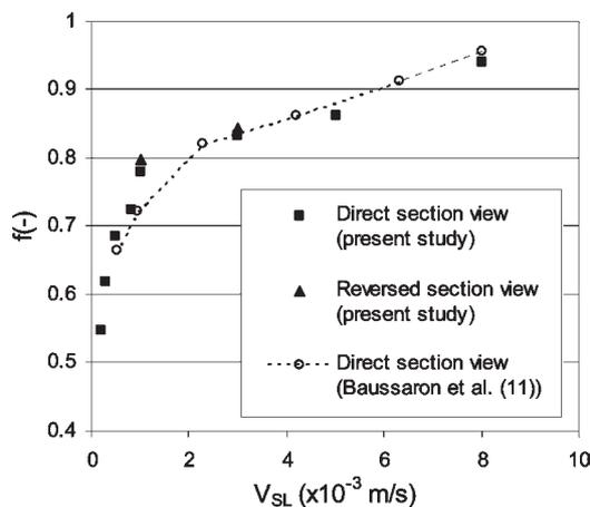
**Figure 3.** Wetting efficiency calculated from direct and reversed section views. Comparison with the results of Baussaron et al.<sup>11</sup> Case 6 from Table 3.
