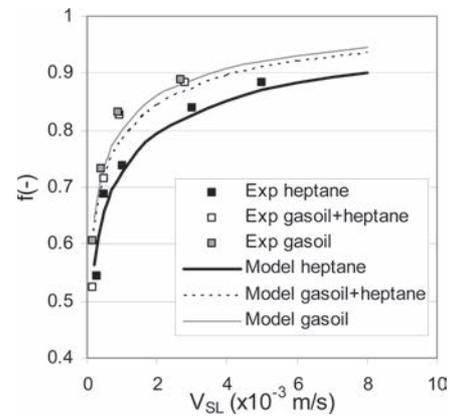
**Figure 4.** Effect of liquid viscosity. Cases 7, 11, and 12 from Table 3.
