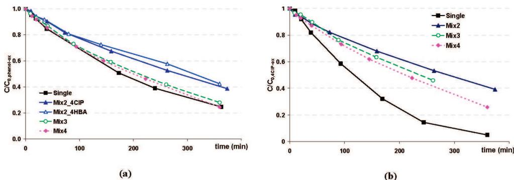
**Figure 3.** Normalized concentration–time profiles of the considered pollutant (single or in mixtures) during batch CWAO over F22, after stabilization of AC activity ( $p_{O_2} = 3.5$  bar,  $T = 150^\circ\text{C}$ , initial concentration of  $1\text{ g}\cdot\text{L}^{-1}$  for each pollutant): (a) phenol, (b) 4-chlorophenol (4CIP) ( $C_{0,ox}$  refers to the concentration after adsorption).
