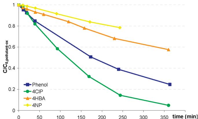
**Figure 2.** Normalized concentration–time profiles of the phenols during batch CWAO on F22, after stabilization of AC activity ( $p_{O_2} = 3.5$  bar,  $T = 150$  °C, initial concentration of 1 g·L<sup>-1</sup> for each pollutant) ( $C_{0,ox}$  refers to the concentration after adsorption).
