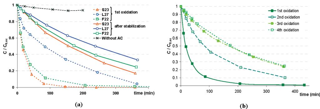
**Figure 1.** Normalized phenol concentration–time profiles during CWAO of phenol ( $p_{O_2} = 3.5$  bar,  $T = 150$  °C,  $C_{ini} = 1$  g·L<sup>-1</sup>): (a) initial and stabilized performance of the investigated carbons, (b) successive oxidations with recycling F22. ( $C_{0,ox} = C_c$  refers to the concentration after adsorption).
