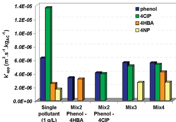
**Figure 4.** Apparent oxidation rate constants ( $k'_{app}$ ) calculated after stabilization of AC activity according to  $R_{pol,app} = k'_{app}C_{pol}$  for the different compound mixtures studied ( $p_{O_2} = 3.5$  bar,  $T = 150^\circ\text{C}$ , initial concentration of  $1\text{ g}\cdot\text{L}^{-1}$  for each pollutant, F22 carbon).
