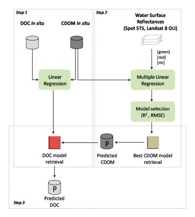
**Figure 2.** Methodological flowchart illustrating the general procedure to retrieve DOC concentrations. The Step 1 corresponds to the computation of the DOC model retrieval and the Step 2 indicates the procedure used to predict CDOM values. The Step 3 shows how the DOC model retrieval is finally used to predict DOC concentrations.
