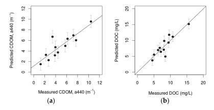
**Figure 6.** (a) Relationship between predicted CDOM at 440 nm (m $^{-1}$ ) and measured CDOM at 440 nm (m $^{-1}$ ) (CDOM<sub>predicted</sub> = 1.15 + 0.76 × CDOM<sub>measured</sub>, R $^2$  = 0.76, p-value < 0.001, RMSE = 1.2). (b) Relationship between predicted DOC in mg/L and measured DOC in mg/L (DOC<sub>predicted</sub> = 0.02 + 0.99 × DOC<sub>measured</sub>, R $^2$  = 0.79, p-value < 0.001, RMSE = 1.4).
