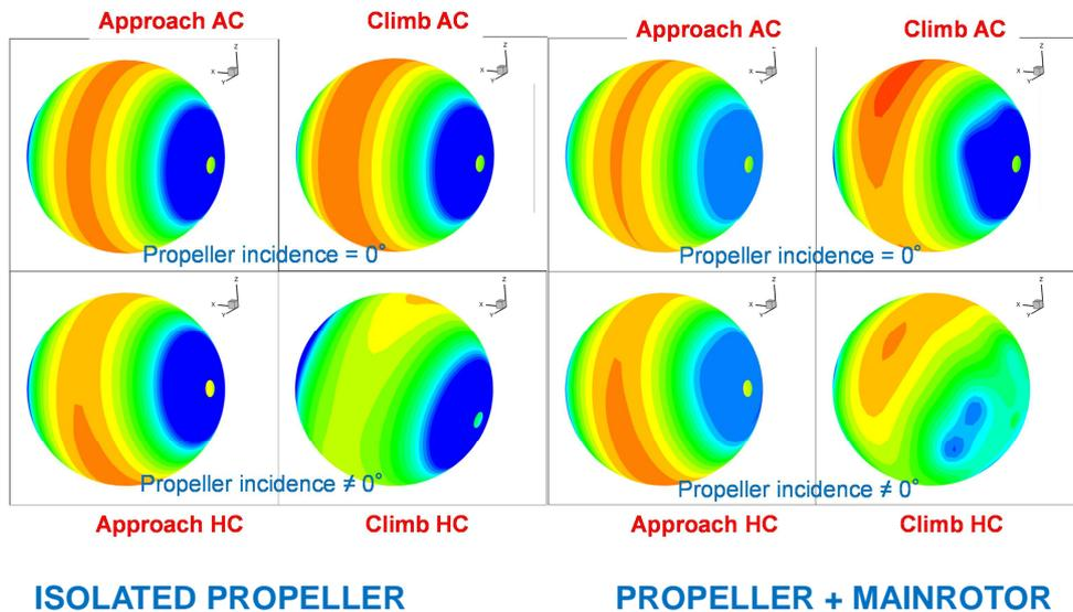
**Figure 6 : Example of acoustic analysis, directivity of the isolated propeller (left) and in the presence of the main rotor (right) depending on the flight configuration. Sphere centered on the propeller, in the near field.**
