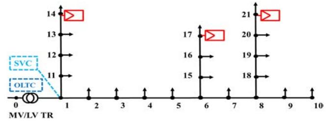
Fig. 8. LV grid under study corresponding to Case #2.
