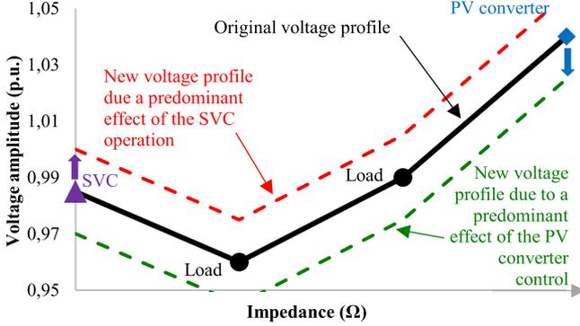
Fig. 5. Example of interaction between SVC and distributed generators.
