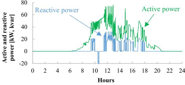
Fig. 9. Daily active and reactive powers from the PV generator in node #18 (CASE#1).
