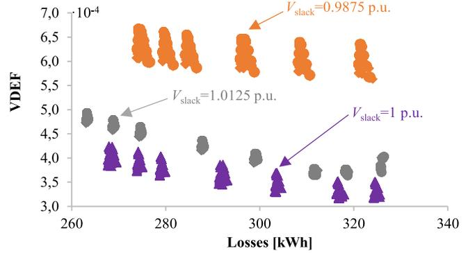
Fig. 12. VDEF-losses chart of the different simulations with OLTC and PV converters controlling voltage (CASE#1).
