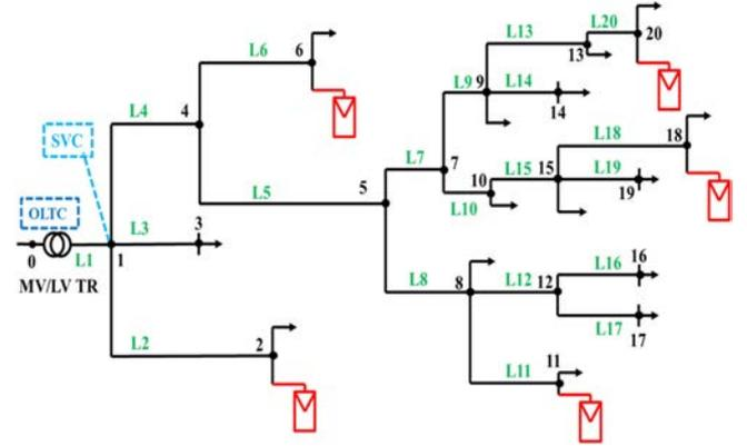
Fig. 7. LV grid under study corresponding to Case #1.
