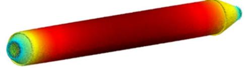
Figure 11: Surface magnetic flux density of a submarine model with 33.298 surfaces elements, 83.245 branches, and 49.947 independent loops, solved in 12 min (i5-6600, 6GB DDR3) with a matrix compression ratio of 89.5 % (ACA).
