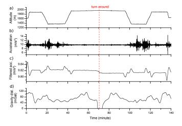
**Fig. 4** Gravity measurements on the Akureyri Snæfellsjökull line. a): Altitude of the plane. b) Raw acceleration measured by the gravimeter. c) Filtered acceleration measured by the gravimeter (4th order low pass Bessel filter of time constant 130 s). d) Estimated gravity disturbance with the 130 s low pass filter.
