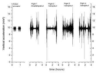
Fig. 3 Top: Flight plan of Iceland gravity campaign. Bottom: Raw vertical acceleration undergone by the atom gravimeter during the motion simulator test and during flights in Iceland. The acceleration has been measured in the sensor head at a rate of  $10~{\rm Hz}$ .
