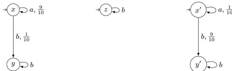
■ **Figure 4** HMMs  $\mathcal{A}_3, \mathcal{A}_4$  and  $\mathcal{A}_5$  (left to right). One cannot classify between  $\mathcal{A}_3, \mathcal{A}_4$ , but they can be attack-classified. On the other hand, one cannot attack-classify between  $\mathcal{A}_3, \mathcal{A}_5$ .
