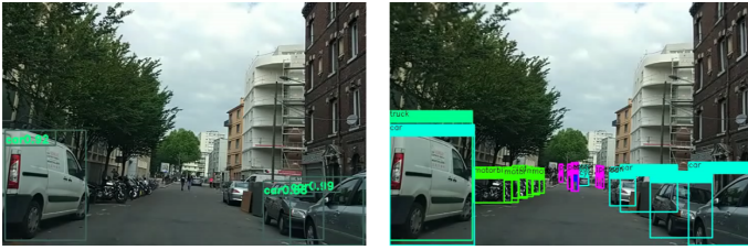
Fig. 1. SSD inference (left) vs YOLO V3 inference (right).
