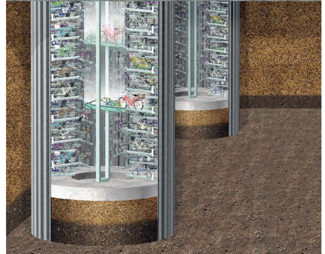
Giken underground eco-cycle parking system, Tokyo
