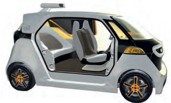
AKKA technology automated demonstrator: the passenger compartment can be transformed into a living room to surf the web, work or watch television, 2013
