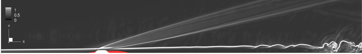
Fig. 6 Instantaneous contours of density gradient magnitude in the centreplane showing transitional flow at the end of the domain, computed with elsA. Red zones showing the recirculation regions.
