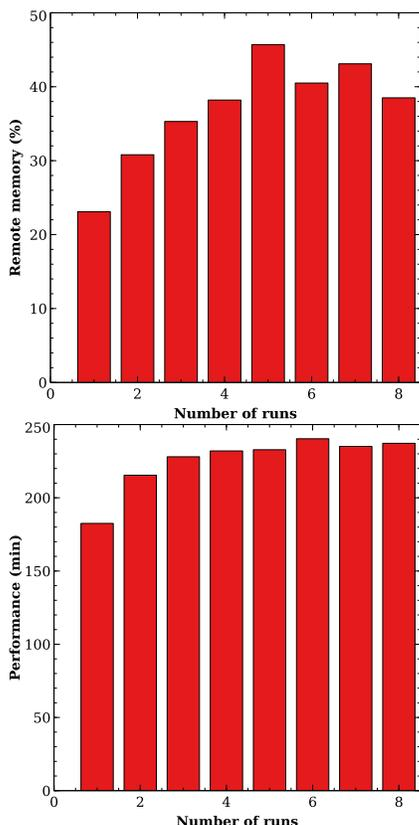
**Figure 2.** The effect of memory flipping, which occurs on I/O intensive applications. The top curve shows the proportion of the VM’s memory which has been remapped on remote nodes after each run. The bottom curve shows the performance of the application after each run.
