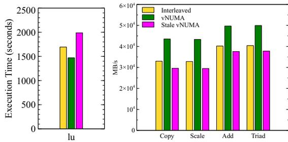
**Figure 3.** Assessment of the negative impact of presenting a stale topology to the VM when vNUMA is used. Evaluation realized using LU from Open MPI 2007 (left, lower is better) and STREAM (right, higher is better).
