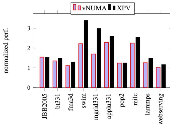
**Figure 5.** XPV implementation efficiency. XPV is compared with vNUMA (implementer by Xen) when no topology change occurs. The performance gap comes from the fact that the implementation of vNUMA by Xen is less optimized than XPV. Recall that the latter does not use any vNUMA code.
