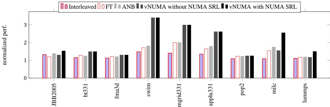
**Figure 7.** vNUMA compared with the state-of-the-art blackbox solutions (higher is better). This experiment also highlight the importance of NUMA policies embedded within the SRL. No topology change is triggered during this experiment.
