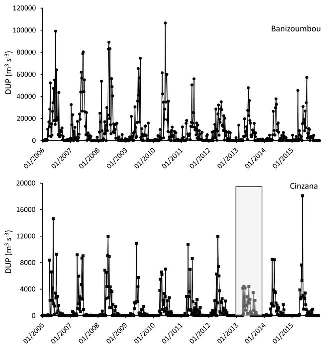
**Figure 4.** Weekly Dust Uplift Potential (DUP) from 2006 to 2015 in Banizoumbou and Cinzana. The gray area in Cinzana corresponds to 2013, a year for which the rate of recorded wind speeds is only 85%.
