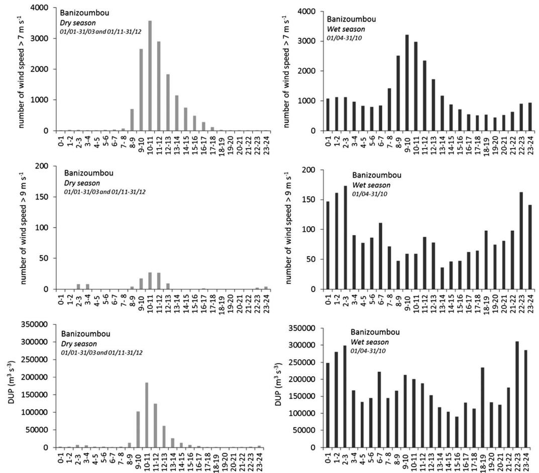
**Figure 3a.** Diurnal cycle of the number 5 min periods of wind speeds  $>7 \text{ m s}^{-1}$  (top),  $>9 \text{ m s}^{-1}$  (middle) and DUP (bottom) in Banizoumbou (Niger). Left: dry season, right: wet season.
