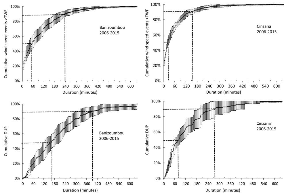
**Figure 2.** Cumulative distributions of the duration of wind speed events  $>TWV$  (top) and of DUP (bottom) for Banizoumbou (left) and Cinzana (right) averaged over the period 2006–2015. The gray envelope corresponds to the minimum and maximum cumulative percentages observed for each class during the 10 years of measurements.
