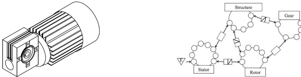
Fig. 12. Drawing of the conveyor electric motor (left) and its FSMo (right)
