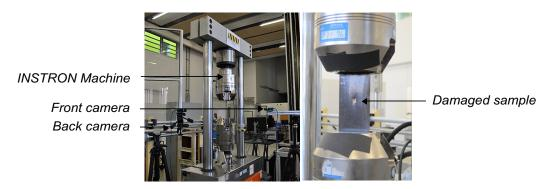
Figure 8: Tensile test on damaged sample
