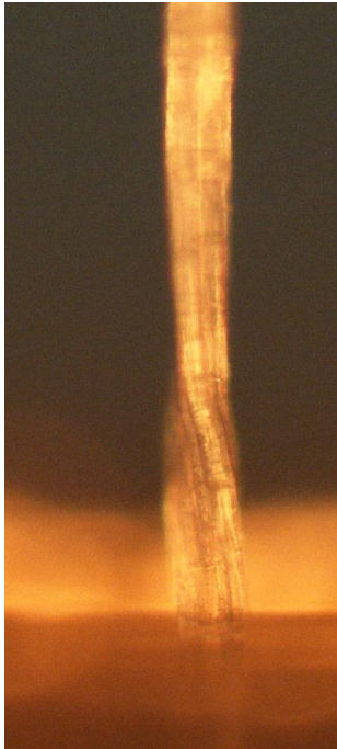
Figure 7: Images of hand-twisted fibres, using polarised light microscopy (a) and scanning electron microscopy (b).
