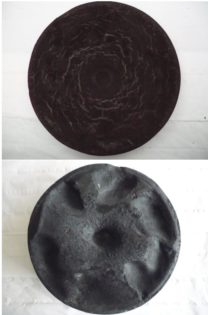
Figure 15: Fuel grain surface after SuperMHYCAS_08 (top) and SuperMHYCAS_10 (bottom) firing tests
