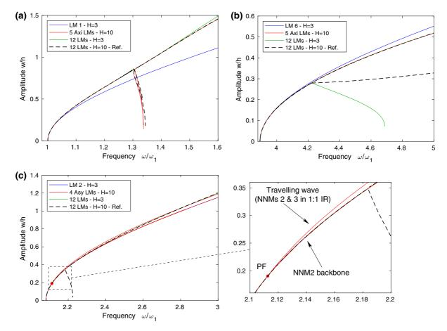
**Fig. 15** Modal convergence with the number of transverse modes of the free responses of the circular plate around some NNMs: **a** first axisymmetric (0,1) (NNM 1), **b** second axisymmetric (0,2) (NNM 6) and **c** first asymmetric (1,0) (NNM 2).
