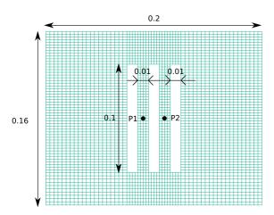
Fig. 16 Geometry and mesh of the structure
