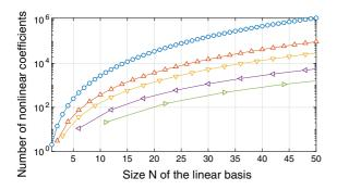
**Fig. 1** Order of coefficients of the ROM as a function of the number N of modes in the expansion basis. ' $\circ$ ':  $N_c$  from Eq. (22); " $\triangle$ ," " $\nabla$ ," " $\triangleright$ ," " $\triangleright$ ," " $\circ$ ":  $N_c'$  from Eq. (24), with  $N=N_u+N_w$  and with, respectively,  $N_u=N_w$ ,  $N_u=2N_w$ ,  $N_u=5N_w$  and  $N_u=10N_w$
