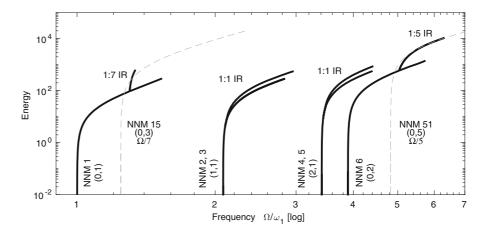
All the NNMs show the same qualitative behavior. First, since both structures are plane, all the NNMs have a hardening behavior, which globally bends the backbone curves toward the high frequencies (indeed, the  $\Gamma^i_{iii}$  coefficients are all positive; see "Appendix D"). Secondly, some internal resonances modify the topology of the backbone curve, which is described more precisely in the next section.
