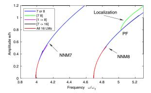
Fig. 20 Modal convergence with the number of transverse LMs retained in the basis, for NNMs 7 and 8. Displacements at the center of one of the beams
