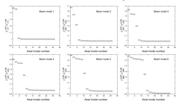
Fig. 4 Evolution of nonlinear beam cubic coefficients  $\Gamma^i_{iii}$  with regard to the number of axial modes retained in the summations of Eqs. (29a), for the first six transverse modes of the beam (1st column of Table 3, i = 1, ... 6)
