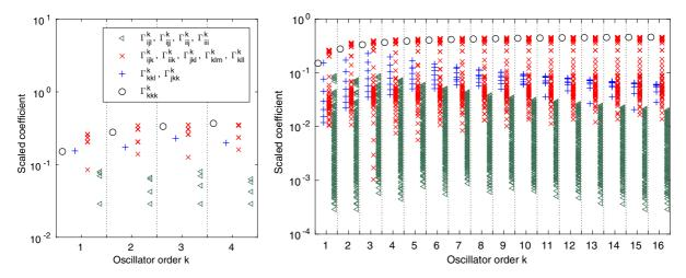
Fig. 18 Scaled cubic coefficients  $\Gamma^k_{ijl}$  of Eq. (43), for the clamped–clamped beam, as a function of k. (left) ROM with 4 bending modes  $i, j, l, k \in \{1, ... 4\}$ ; (left) ROM with 16 bending modes  $i, j, l, k \in \{1, ... 16\}$
