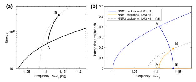
**Fig. 10** Topology of the 1:5 internal resonance of NNM1 with NNM3 of the clamped–clamped beam. **a** Zoom of the FEP of Fig. 8 and **b** harmonics amplitude of NNM1 (H1 of LM1 in blue
