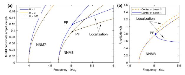
**Fig. 19** Response of the two LMs reduced-order model. a Convergence as a function of the number of harmonics components of the modal coordinates  $q_7$  and  $q_8$  on the backbones of NNMs
