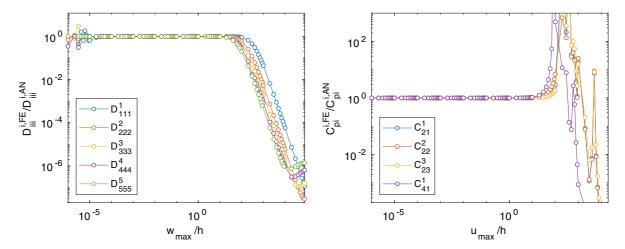
**Fig. 3** Sensitivity of cubic coefficient  $D^k_{kkk} \equiv b^k_{kkk}$  to the maximal prescribed transverse displacement of mode i (left) and of quadratic coefficient  $C^i_{pi} \equiv a^i_{pi}$  to the maximal prescribed axial displacement of mode p (right). Clamped–clamped beam FE model
