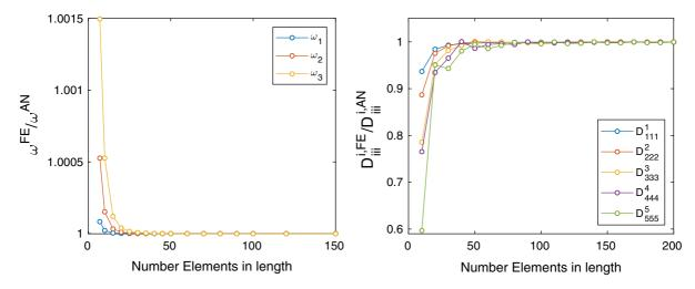
**Fig. 2** Convergence of the first eigenfrequencies  $\omega_k$  (left) and of the cubic coefficients  $D_{kkk}^k \equiv b_{kkk}^k$  (right) as a function of the number of FE in the length of the beam, computed by the FE
