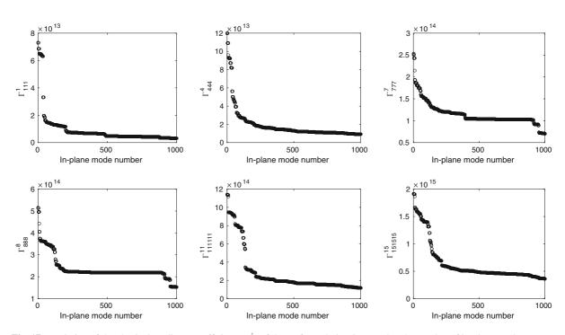
Fig. 17 Evolution of the physical nonlinear coefficients  $\Gamma^i_{iii}$  of the perforated plate in regard to the number of in-plane modes
