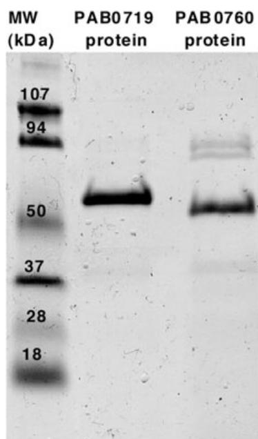
**Fig. 2.** Electrophoretic analysis of the purified recombinant PAB0719 and PAB0760 proteins. An SDS-PAGE was performed using 10% acrylamide gels, and the proteins were stained by Coomassie blue. Lane 1, molecular weight markers in kDa; lane 2, PAB0719 protein (49 kDa); lane 3, PAB0760 protein (48.6 kDa). Both proteins were purified by Ni-affinity chromatography.
