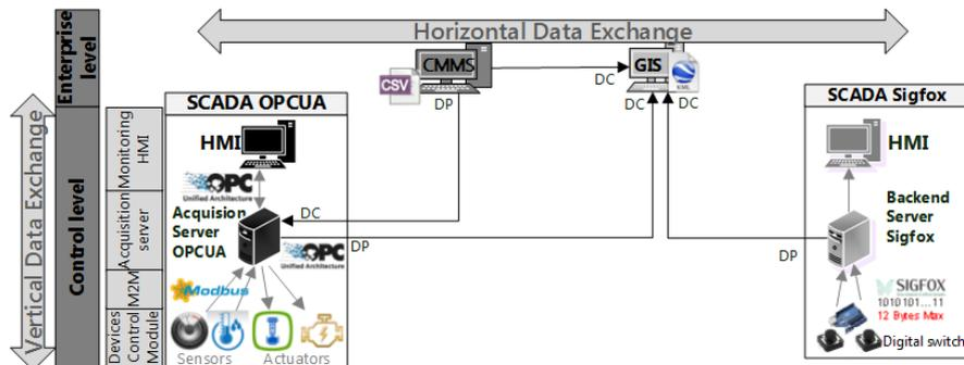
Fig. 1. Data Flow and exchange between heterogeneous systems
