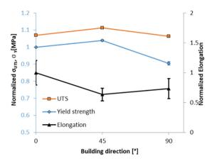
Fig. 9. Tensile behaviour of the investigated alloy fabricated with the three building directions [50].
