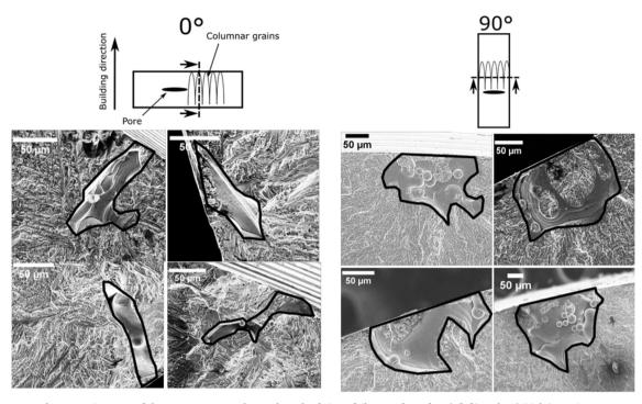
Fig. 12. Anisotropy of the pore geometry observed on the fatigue failure surfaces for 0° (left) and 90° (right) specimens.
