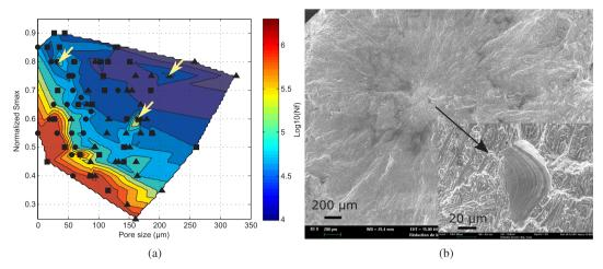
Fig. 16. (a) Generalized Kitagawa-Takahashi diagram or the  $S-\sqrt{area}$  - $N_f$  map for all pores. The arrows indicate specimens for which crack initiation occurred from internal pores and (b) SEM images showing crack initiation from an internal pore [50].
