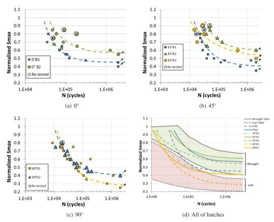
**Fig. 10.** Wöhler curves for all of specimen batches: (a) 0° batches, (b) 45° batches, (c) 90° batches and (d) superposition of the Stromeyer theoretical curves of all batches. The arrows indicate the run-out specimens. The fatigue data bands for wrought and cast TA6V is documented in [35].
