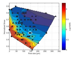
**Fig. 18.**  $S - \sqrt{area} - N_f$  map for only surface lack-of-fusion pores (i.e. without internal pores and spherical gas pores); circular dots = 0° specimens, square dots = 45° specimens, triangle dots = 90° specimens.
