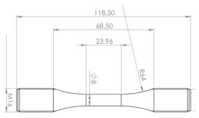
Fig. 2. Final geometry of the fatigue specimens [50].
