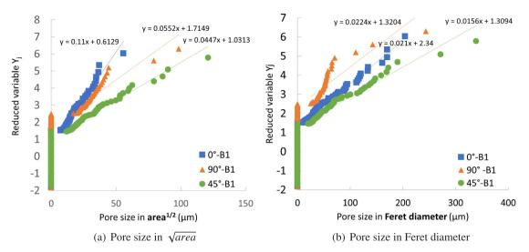
Fig. 7. Pore size distributions measured on polished samples of the three batches  $0^{\circ}$ -B1,  $45^{\circ}$ -B1 and  $90^{\circ}$ -B1. The observation planes are perpendicular to the specimen axis as shown in Fig. 6.
