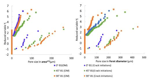
Fig. 13. Comparison of the pore size distributions obtained from observations on polished samples using optical microscopy (square data points labelled "OM") and on failure surfaces(circular data points labelled "Crack initiations").
