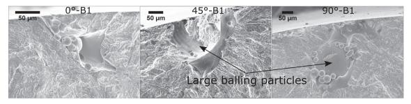
Fig. 11. Fatigue crack initiation site observed on a 0° (left), 45° (middle) and 90° (right) specimen [50].
