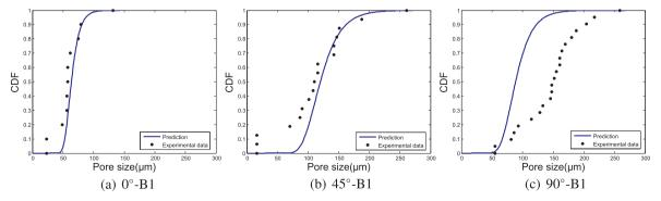
Fig. 14. Correlation between the maximum pore size distributions predicted from the metallographical pore size characterization and the pore size distributions measured on the crack initiation sites.
