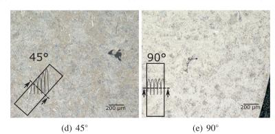
**Fig. 4.** (a) to (c): observation planes parallel to the building direction; (d) and(e): observation planes perpendicular to the specimen axis for 45° and 90° specimens.
