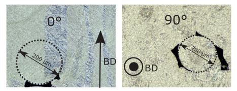
Fig. 5. Pores formed by the balling effect observed on a 0° (left) and 90° (right) specimen.
