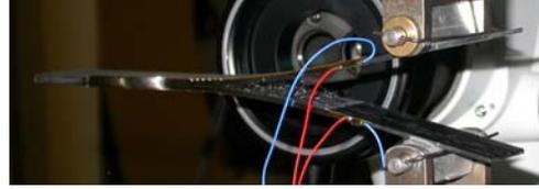
Figure 2. Mode I testing and opened sample.
