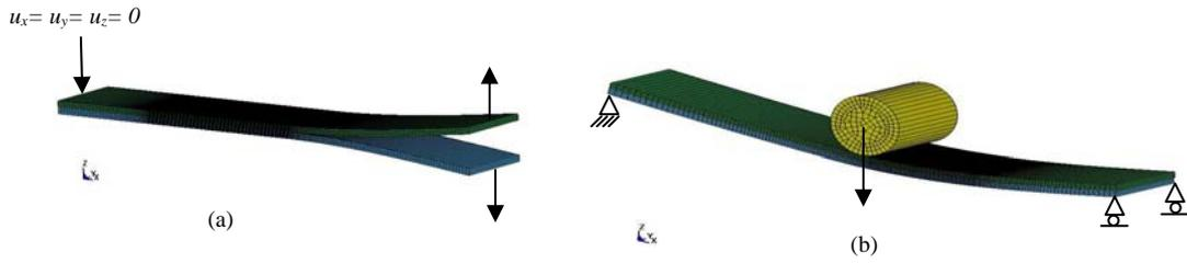
Figure 3. Numerical models (a) DCB and (b) ENF.
