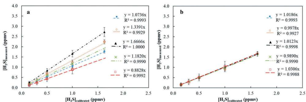
**Figure 2.** Comparison between measured and calibrated H<sub>2</sub>S concentrations for 5 humidity levels and its respective linear regression (dotted lines): 0.01%vol of H<sub>2</sub>O (●); 0.50%vol of H<sub>2</sub>O (○); 2.00% vol of H<sub>2</sub>O (▲); 3.50%vol of H<sub>2</sub>O (✕) and 5.00%vol of H<sub>2</sub>O (□). (a) Considering the ionisation rate coefficients values shown in Table 2. (b) Considering the apparent product formation rate after correcting according to water amount.
