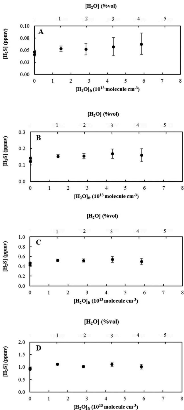
**Figure 5.** Uncertainty related to H<sub>2</sub>O and H<sub>2</sub>S levels of concentration. The H<sub>2</sub>S concentration axis is limited to the double of the calibrated concentration to express the relative error (calculated as the standard deviation of a 400 s measurement time analysis by SIFT/MS). (a) 0.05 ppmv of H<sub>2</sub>S. (b) 0.15 ppmv of H<sub>2</sub>S. (c) 0.5 ppmv of H<sub>2</sub>S and (d) 1.0 ppmv of H<sub>2</sub>S.
