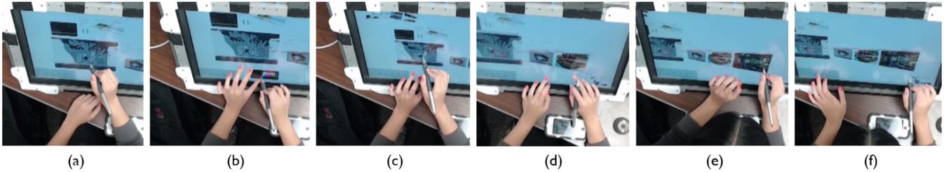
**Figure 1. Hovering interstice sequence:** (a) LH rests on the desk (Rested); (b) LH lifts and performs a gesture (activate ink properties tool); (c) LH is Hovering near the surface without contact, RH draws ink strokes; (d) LH and RH bimanually zoom and pan to situate interaction; (e) RH draws additional ink strokes, LH is Hovering; (f) LH swipes on the Hotpad to undo an erroneous ink stroke.
