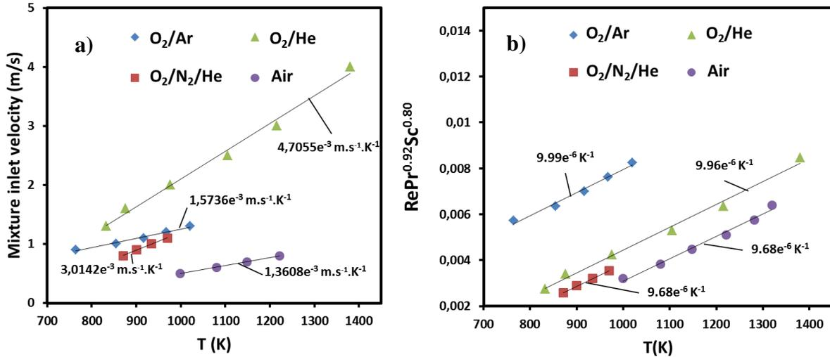
Figure 2: a) Temperature stabilization of stoichiometric CH<sub>4</sub> flames as a function of mixture inlet mean velocities for different diluents; b) Temperature stabilization as a function of  $RePr^{0.92}Sc^{0.80}$ .
