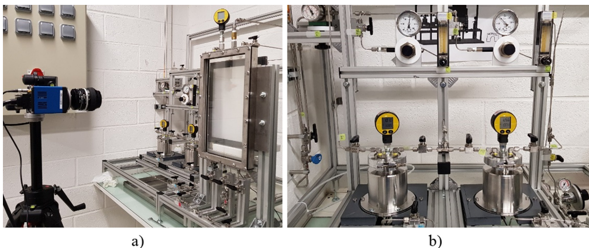
Fig. 3. Pictures of the experimental set-up: (a) Panoramic view. (b) Gastight vessels made of stainless steel (one containing the cleaning solution and the other the initial Cu(I)-complex solution).
