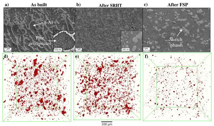
**Fig. 1.** SEM micrographs depicting the microstructural features and 3-D X-ray synchrotron tomography reconstructions showing porosity of SLM AlSi10Mg as built (a,d), after SRHT at 300 °C during 2 h (b,e) and after FSP at 1000 rpm rotational speed and 500 mm/min traverse speed (c,f)
