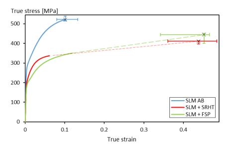
**Fig. 2.** Representative tensile true stress - true strain curves of SLM AlSi10Mg AB, SRHT and FSP (out of 6 tested samples for AB and 3 for SRHT and FSP)
