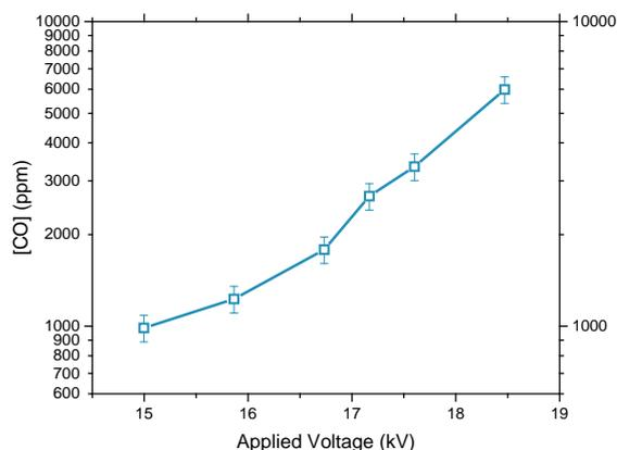
Figure 3: CO density as a function of the applied voltage in log-log scale. The gas flow is 500 sccm of He with 1% of CO<sub>2</sub> and the repetition frequency is 5kHz.
