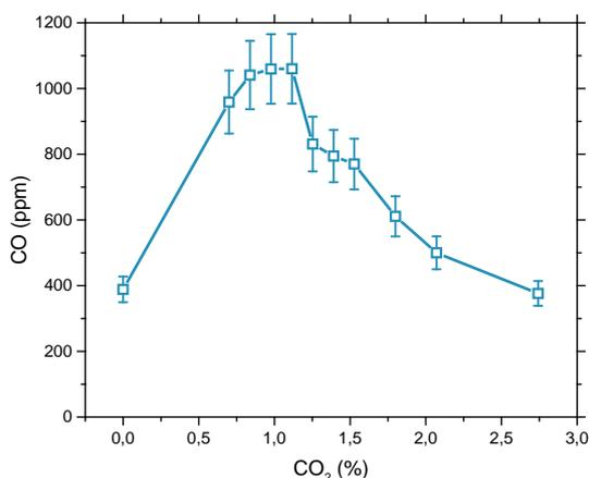
Figure 2: CO fraction as a function of the CO<sub>2</sub> percentage. The total gas flow is 500 sccm. The applied voltage is 15kV, and the repetition frequency 5kHz.
