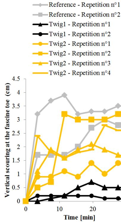
Figure 12: Scouring depth below the fascine with and without twigs (twigs 1 = 0.7–1.4 mm and twigs 2 = 0.4 mm).
