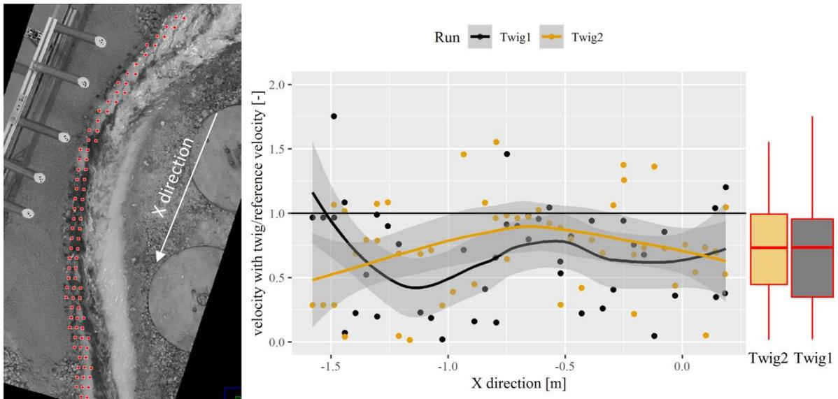
Figure 14: Velocity ratio between the twig experiments and the referent experiment with no protection. Thick stiff twigs (twig1) reduce velocity more than thin twigs (twig2)
