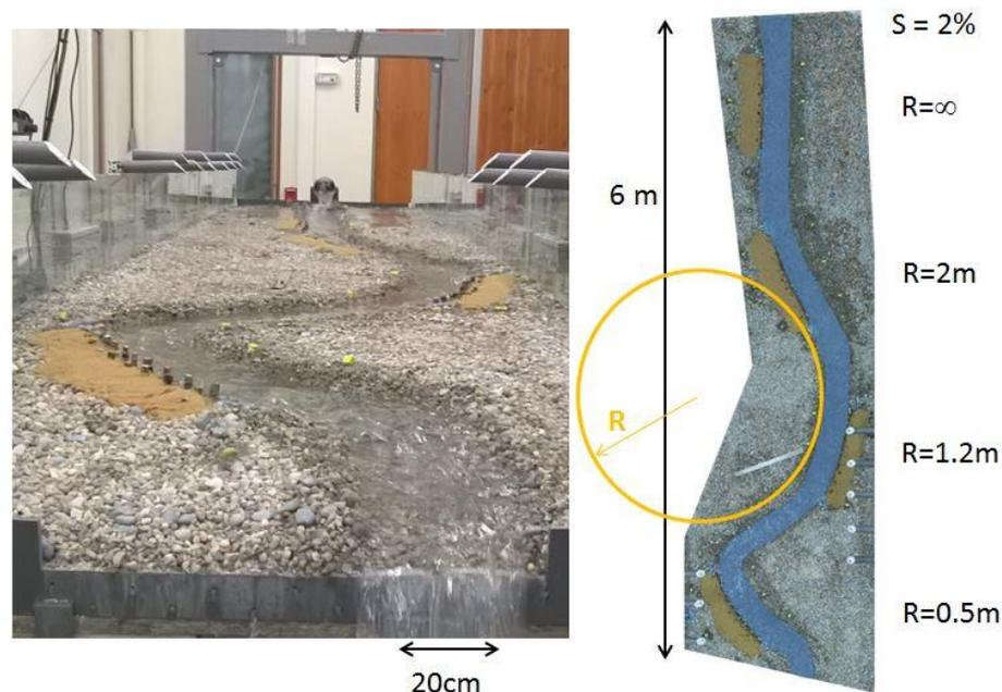
Figure 6: Set-up for the first set of experiments with a fixed flume bed and four curvature radii
