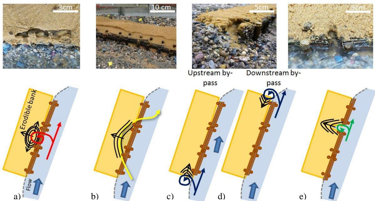
Figure 8: Five main failure modes observed during the first set of experiments: a) toe erosion, b) upper bank surface erosion, c) fascine upstream by-pass, d) fascine downstream by-pass and e) fascine bundle discontinuity
