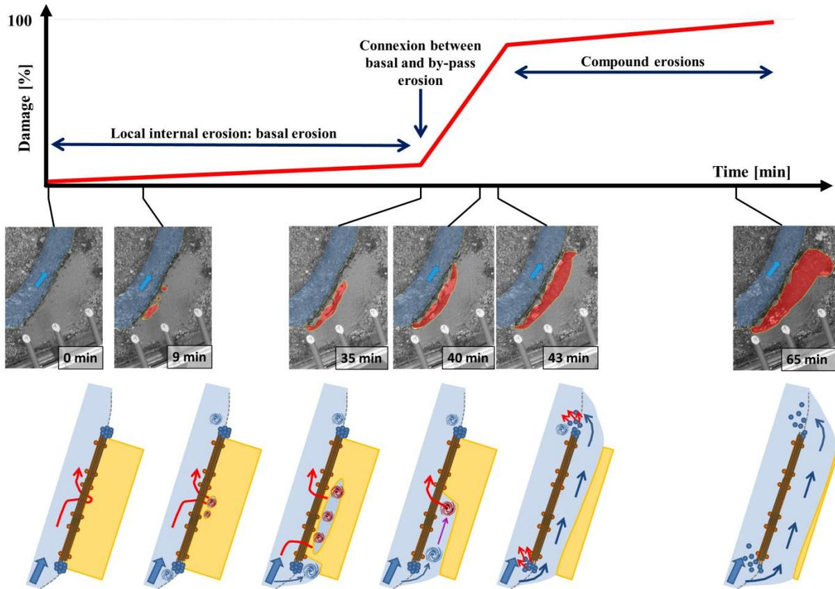
Figure 9: Main steps involved in full failure of the structure over time. Flume aerial pictures (in red: extent of bank erosion) and synthesis sketches. Local erosion creates weaker points and local damage. Damage rate sharply increases when by-pass erosion connects with existing points, enabling the flow to pass behind the protection, get loaded with bank material and extend further.
