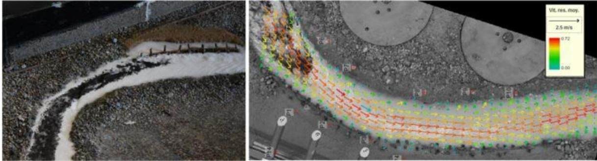
Figure 5: Example of flow seeding and velocity field measured with LSPIV (Large-Scale Particle Image Velocimetry)
