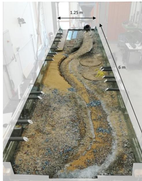
Figure 7: Set-up for the second set of experiments with a mobile flume bed and one curvature radius; the lateral bars attached to the walls support the targets used by photogrammetry
