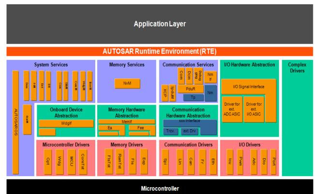
Figure 6: AUTOSAR Layered Architecture (not all modules are shown here)
