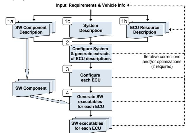
Figure 5: Implementation / Integration Process as defined by AUTOSAR
