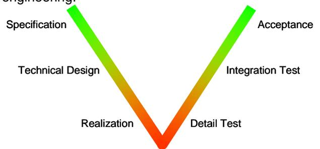
**Figure 3: Main generic objectives of the V model**
