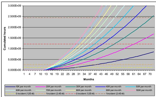
For example, it will take 16 months for a candidate introduced in the field with a production of 40 000 parts per month to be proven in use with regard to a safety goal ranked ASILC in case no incident is observed. It will take 21 months in case one incident is observed.
