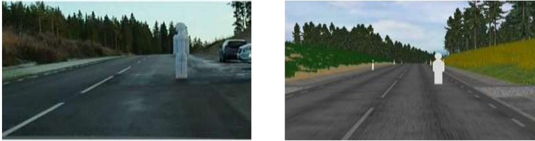
**Figure 30: Test Track and Virtual world, critical object spawn position.** predefined The actions were taken in the following order (1) distraction task, (2) spawn of critical object, (3) warning, and (4) intervention. Each set of TTC triggers contains a reference TTC for each action, and two such sets were used in the simulator experiment (Table 7.)
