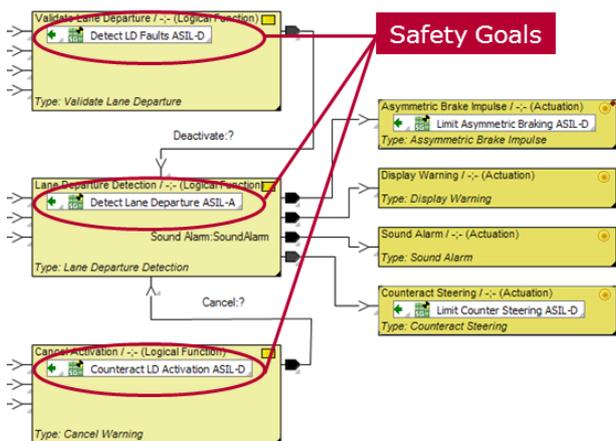
**Figure 4 Vitalization: Allocation of safety goals to system safety concept**
