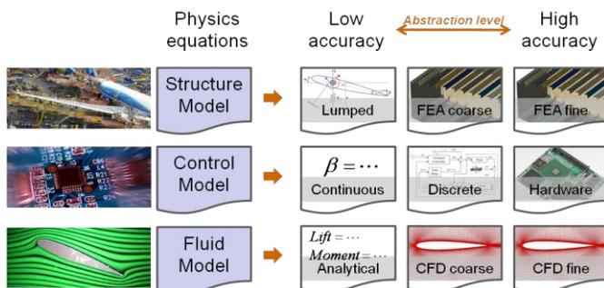
Multiple hierarchical abstractions in the RFLP-based design product structure are available for use in simulation models.
