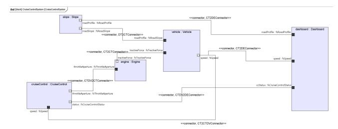
Figure 2 – Cruise Control Internal Block Diagram
